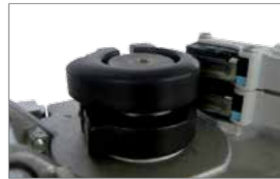
Limit switch with high precision regulation
